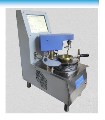
**AutoFlash-92(ver 2.0)** is programmable fully automated micro controller based standalone Cleveland Open Cup Flash Point Analyzer conforming to standard ASTM D92, ISO 2592, IS 1448 (P:69) & IP 36.
